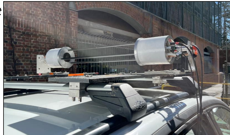
Experimental setup of the open-path NH 3 sensor on the mobile platform at Princeton University
